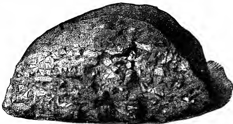
FIG. 91.—FRACTURED SURFACE OF CONNECTING ROD.
